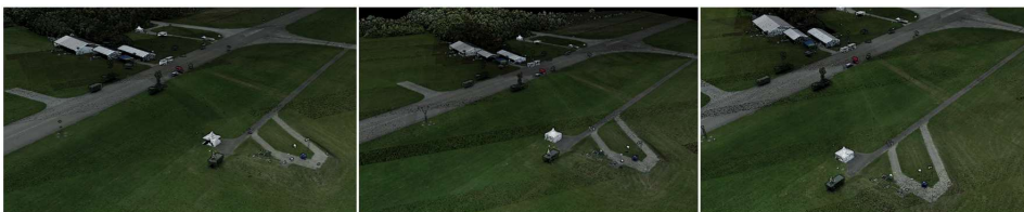
Fig. 7 Results of lidar point cloud overlayed with photogrammetry: The 100 m altitude flight, 50 m altitude flight, and a combination of both datasets.
