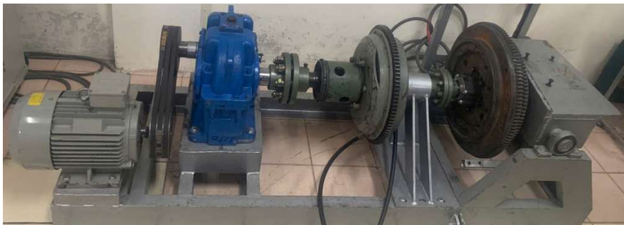
Fig. 6 Experimental setup for accelerated testing of friction disc
