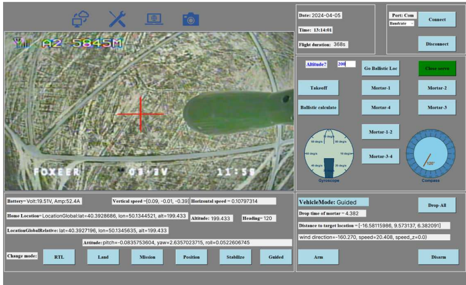
Fig. 6 Final version of mission software interface showing full munition control, sensor visualization
