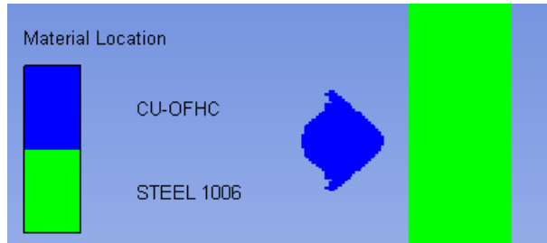
Fig. 2 Simulation of EFP impact on steel plate
