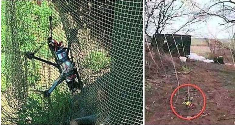
Fig. 4 Netting and curtains to protect against FPV drones
