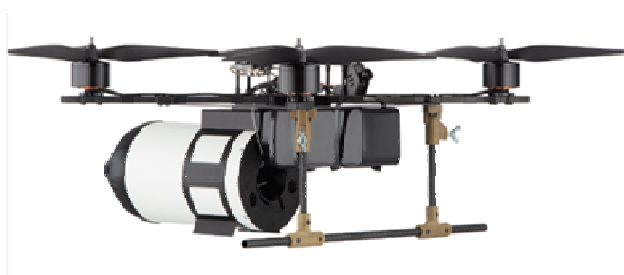
Fig. 5 Appearance of a UAV controlled via fiber optic communication lines
