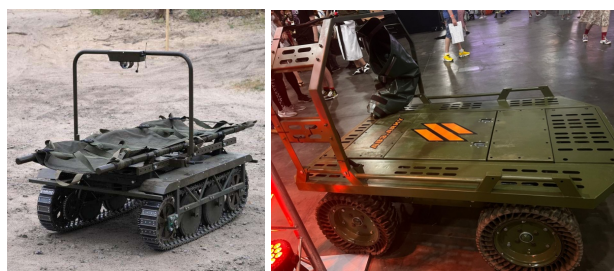
Fig. 2 Evacuation unmanned ground vehicles on different chassis
