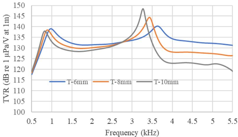
*Fig. 7 Effect of piezoceramic ring thickness on TVR*
