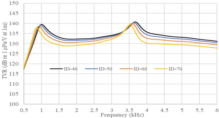
Fig. 5 Effect of piezoceramic ring inner diameter on  $TVR$
