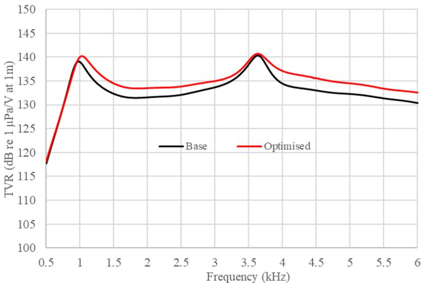
Fig. 10 TVR of the base model and optimised transducer model
