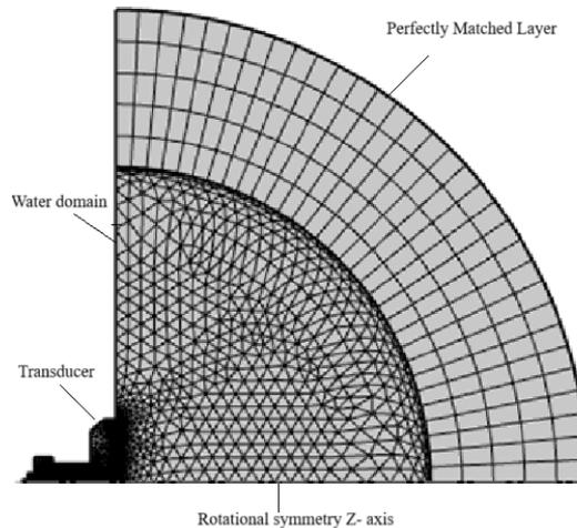
*Fig. 2 2D axisymmetric model of the Tonpizl transducer*
