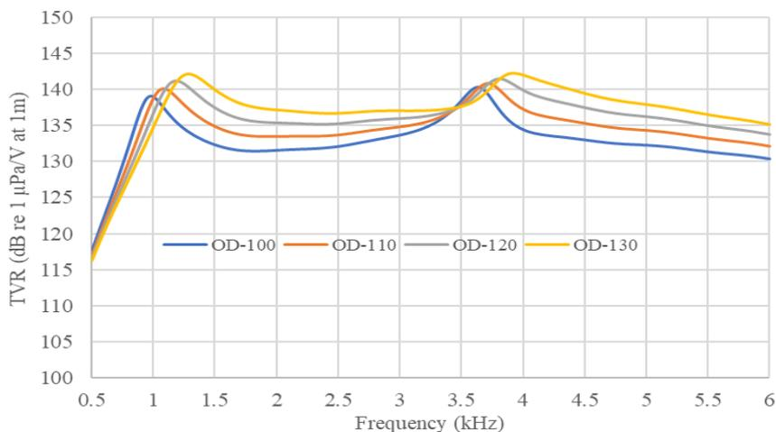
Fig. 6 Effect of piezoceramic ring outer diameter on  $TVR$
