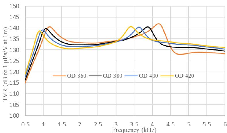
*Fig. 8 Effect of head mass outer diameter on TVR*
