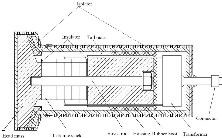
*Fig. 1 Schematic of a Tonpiliz transducer.*
