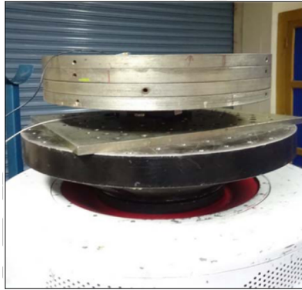
Fig. 3 Vibration test of mount on exciter head with 152 kg dead load in z axis [9]
