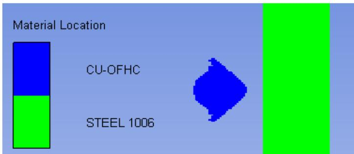
*Fig. 2 Simulation of EFP impact on steel plate*
