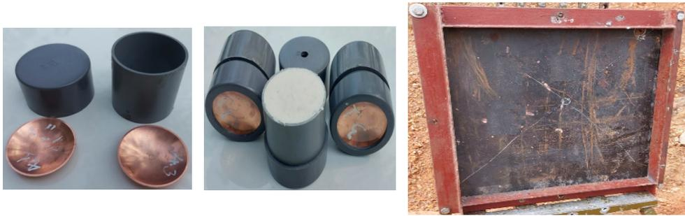
Fig. 3 EFPW and steel target
