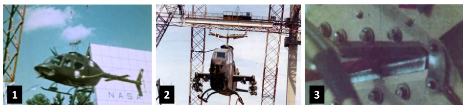
Fig. 6 Large-scale tests on a swing test facility (Ford Eustis, Virginia, U.S.) in 1980 and 1982: (1) the Bell OH-58A Kiowa, (2) the Bell AH-1S Cobra, and (3) close-up view of the cutter cutting the wire [30-32]
