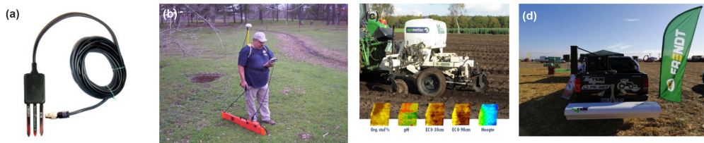
Fig. 3 SMTE sensor of moisture content, temperature and soil electric conductivity – a; Geonics EM-38 for measuring soil electromagnetic conductivity – b; Veris sensor system for measuring acidity (pH), percentage of organic matter at the depth of growth (0-30 cm) and in the root zone (0-90 cm) – c; Topsoil Mapper to determine structure, moisture availability, compaction and optimal loosening depth – d
