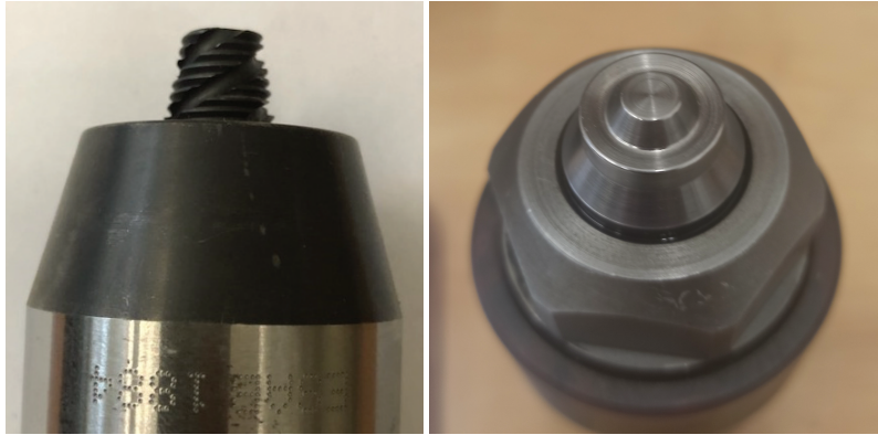
Fig. 1 Welding tools: MX Triflute for joining aluminum (left) and W-La tool for joining titanium (right)
