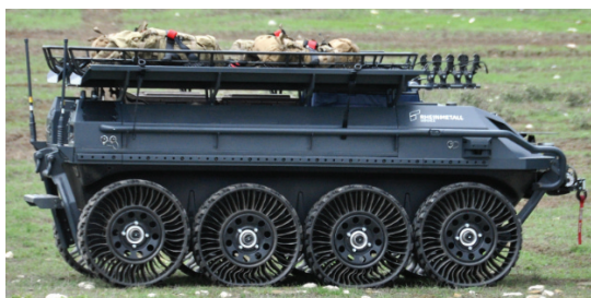
Fig. 8 The UGV Mission Master SP fitted with special wheels using the Airless Tire System [24]
