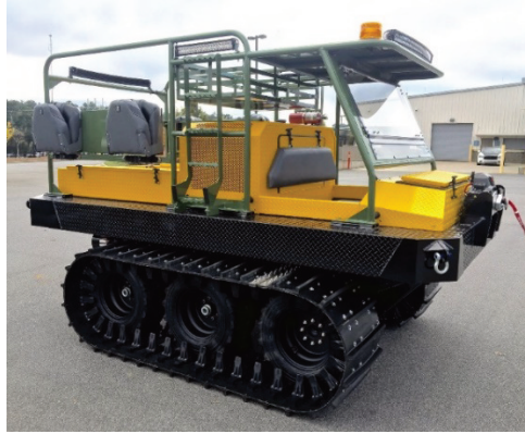
Fig. 6 The basic platform of the UGV SMSS, the ATV Land Tamer equipped with tracks [20]
