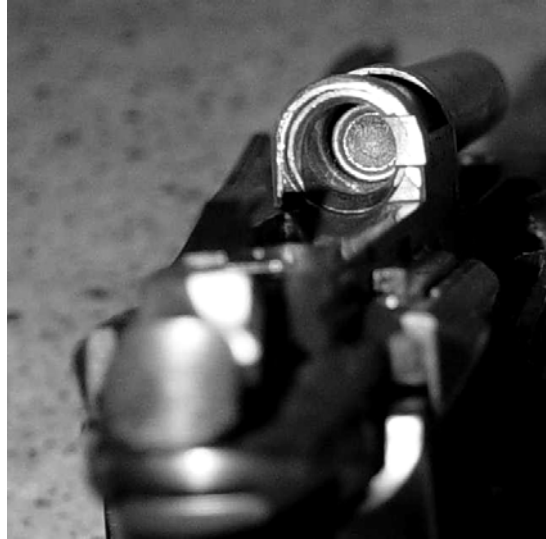
Figure 6 – View into cartridge chamber with projectile impressed into forcing cone
