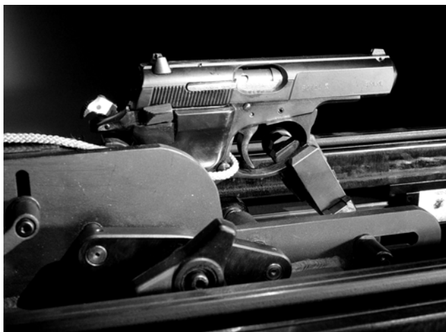
Figure 5 – Loaded gun placed on universal firing bench (Prototypa Brno, a. s.)
