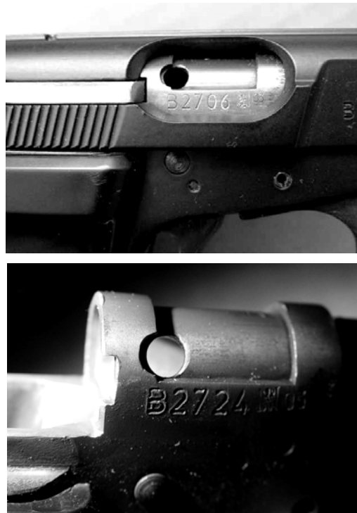
Figure 4 – Detail of the ejection window and the back part of the barrel of the pistol CZ 83 PA Rubber with adjusted cartridge chamber (discharge hole is placed on the transition of the weakened part of the barrel wall into full part)
