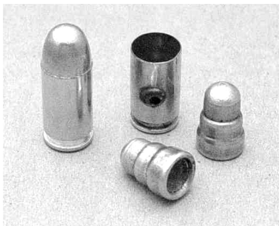
Figure 8 – Cartridge 9 mm Browning court (on the left cartridge before firing, on the right fired cartridge case with a circular hole in its body and two deformed projectiles after their extraction from the barrel)
