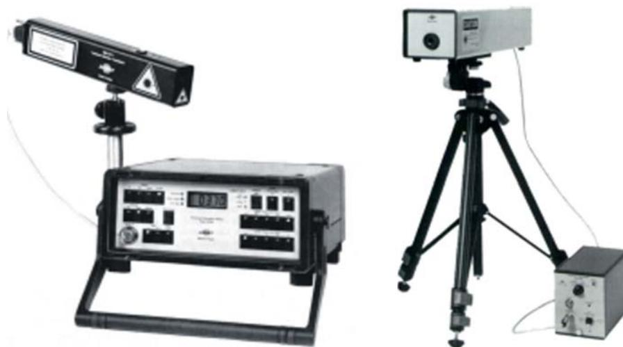
**Figure 5** Laser torsional vibration meter B&K Type 2523 (left) and Laser vibration meter B&K Type 3544 (right)
