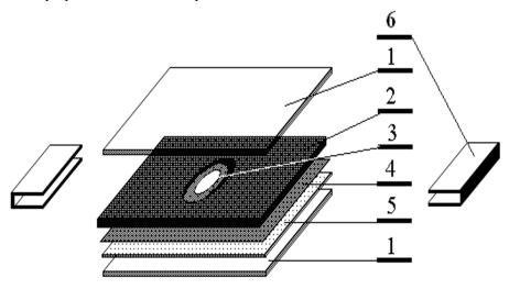
Fig. 1 The breakthrough time measuring utility ready to be put into a thermostat
