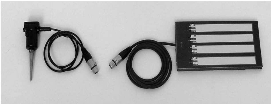
Fig. 1. The Picture of a geophone build in a case PE 3-D (left), Piezo Film type LTD (right).
