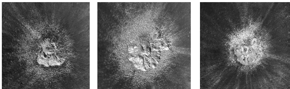
Fig. 3 Details of the front side of the plate of thickness 10 mm after the first bullet impact (left), third bullet (middle) and the fifth bullet (right) of the calibre 308 Winchester shot in the same place – experiment No. 3, shot No. 6
