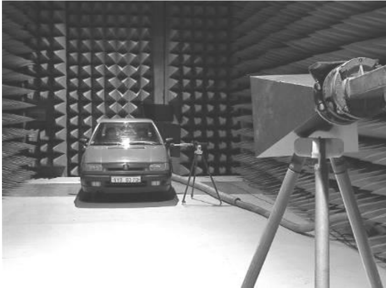
Fig. 13 Stopping the car engine with HPM irradiation use (HPM 3 GHz)
