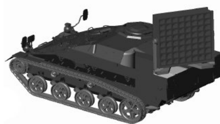
Fig. 4 HPM system with antenna array installed on a tank [2]
