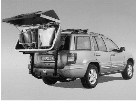
Fig. 5 Electromagnetic System for Selective Car Stopping [2]
