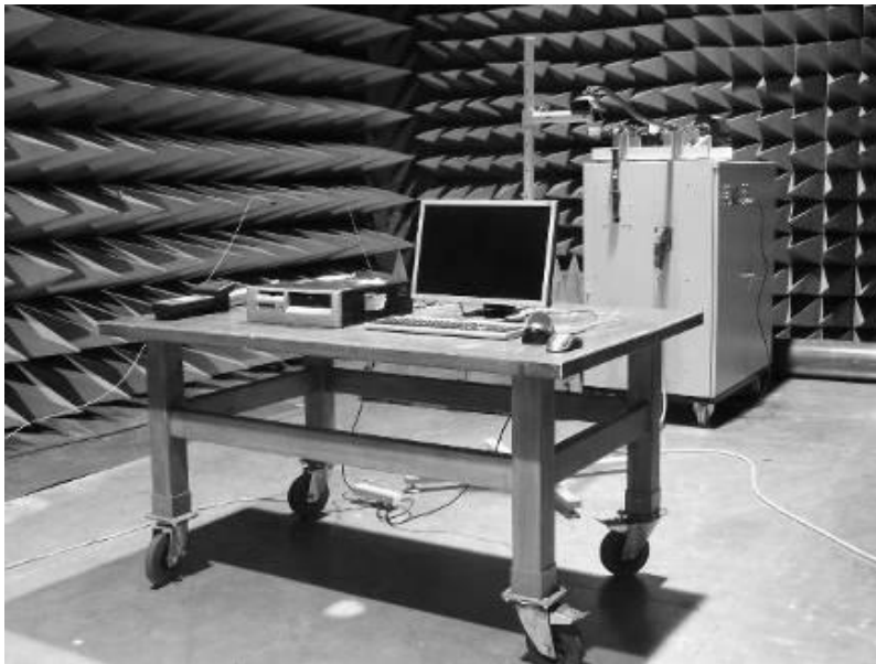
Fig. 14 PC setup irradiated with HPM 9 GHz
