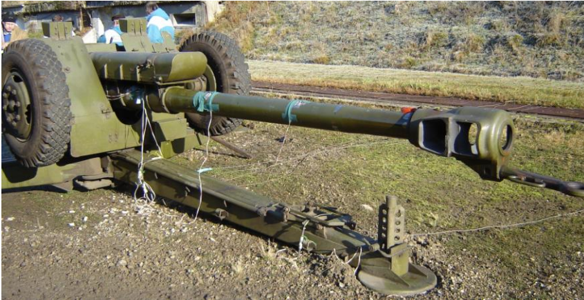
Fig. 1 122 mm H D-30 gun provided with strain gauges
