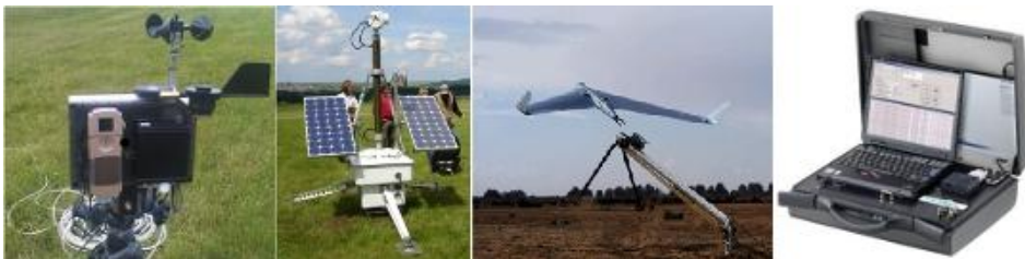
Fig. 4 ESS base equipment (from left): meteorological sensors with INCA modem, unmanned ground station (UGS), unmanned aerial vehicle (UAV), IMSI catcher
