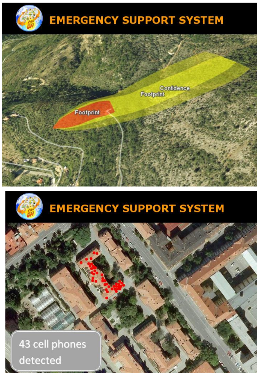
Fig. 5 ESS Portal as the visualization of the Emergency Support System (from top): view on the ALOHA model, results of people presence calculation (obtained from IMSI catcher)
