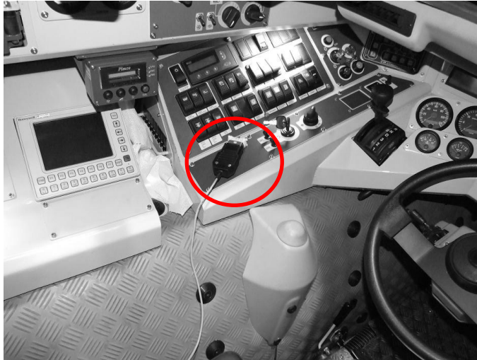
Fig. 3 Data reading by means of diagnostics interface built in the dashboard of AMV Rosomak [personal photo]
