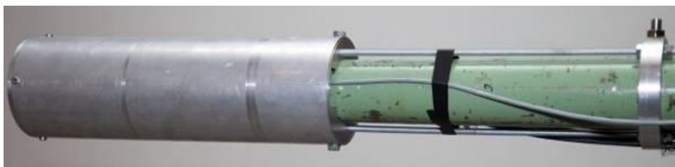
Fig. 10b Final form of protection of gauges, mounted on the barrel
