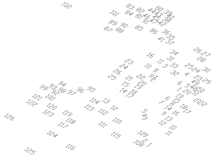
Fig. 5 Graphic projection of spatial coordinate list of detailed survey points
