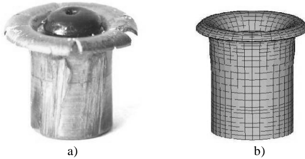
Fig. 11 Comparison of experimental (a) and simulation (b) deformed bullet
