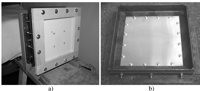
Fig. 4 Scheme of fuselage structure assembly (a) and mounting of the duralumin fuselage skin on experimental frame (b)
