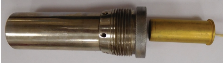
Fig. 3 Assembly of breech module with the power cartridge
