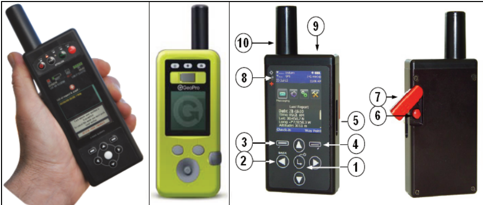
Fig. 14 Iridium Personal Satellite Trackers [14]
