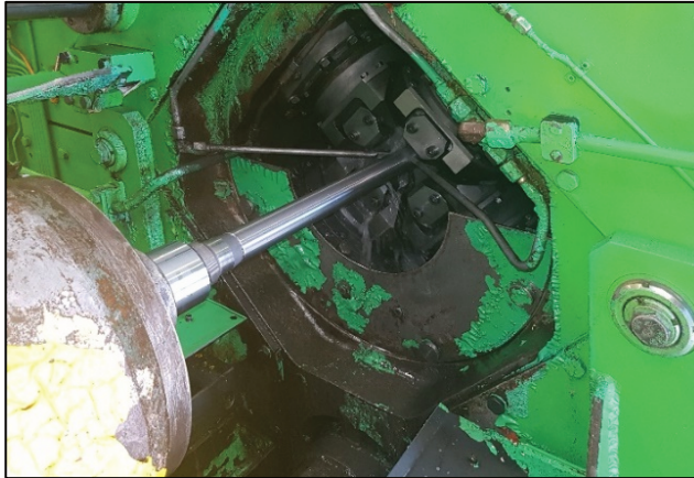
Fig. 2 Barrel blank forging on GFM SHK10 machine
