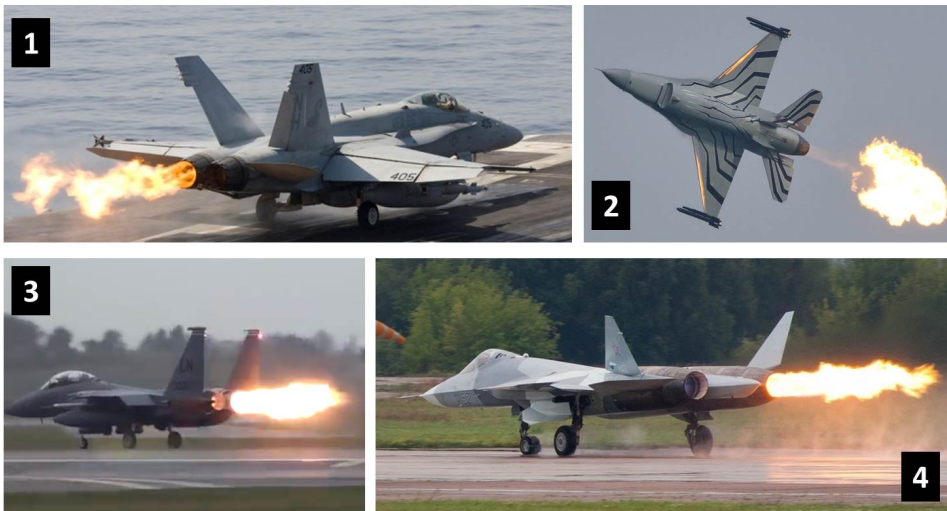
Fig. 2 Examples of surging engines in foreign military jet fighters: (1) F-18 C (2009), (2) F-16 A (2016), (3) F-15 E (2014), (4) Su-57 (2011) [5]
