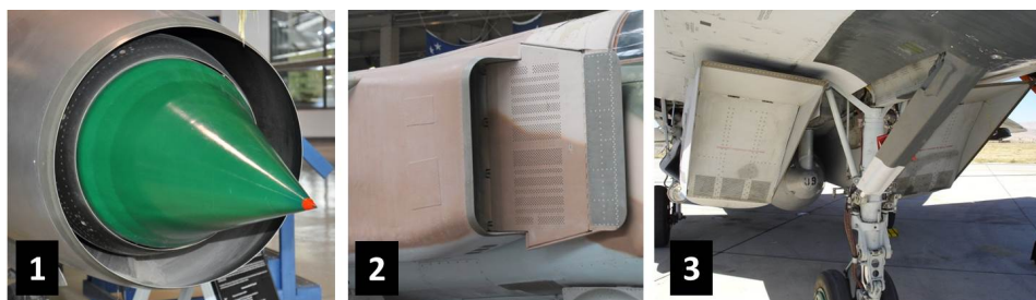
Fig. 4 Examples of various inlet designs: (1) MiG-21, (2) MiG-23, (3) MiG-29 [5]
