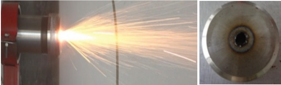
(a) Steel ally nozzle burning during firing
