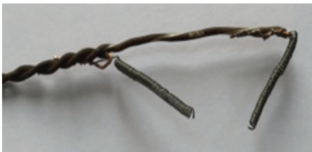
(c) Igniter failure
