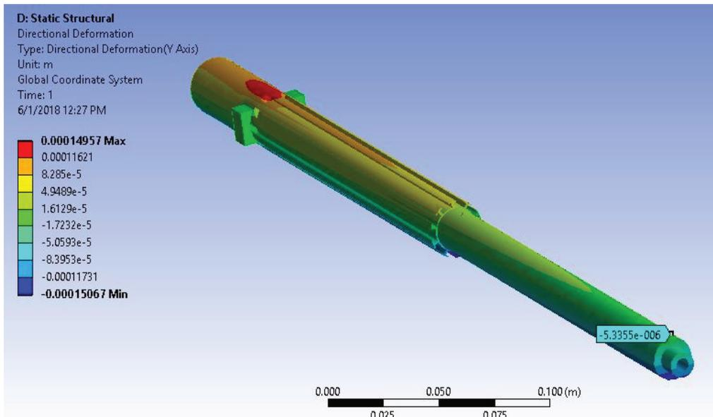
Fig 9 Directional deformation towards the ground due to gravity in modified T-section finned barrel. The probe at the muzzle end shows the numerical value for the maximum deflection at the muzzle
