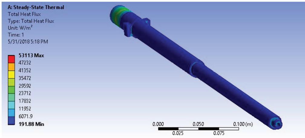
*Fig. 6 Heat dissipation in plain thick profile barrel*
