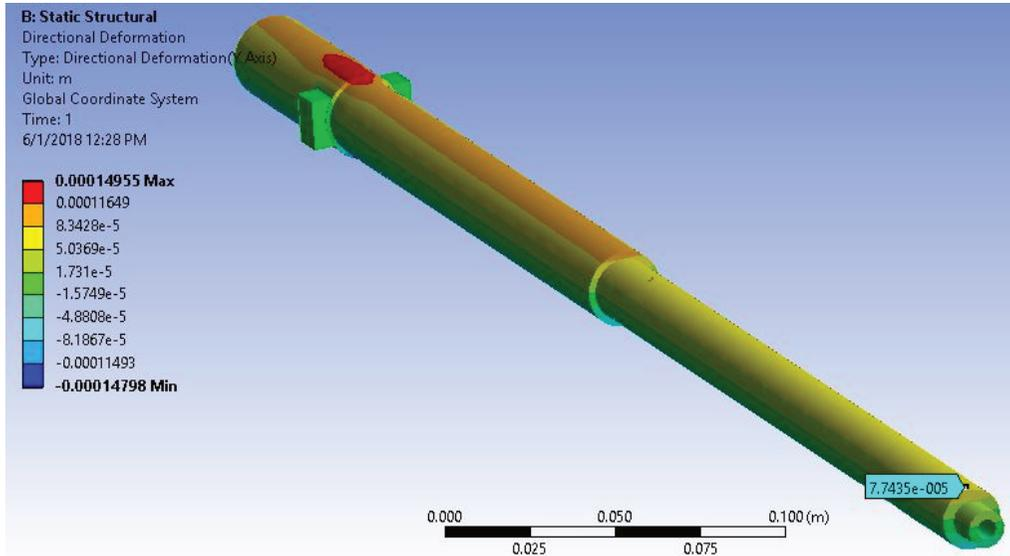
Fig. 8 Directional deformation towards the ground due to gravity in plain barrel. The probe at the muzzle end shows the numerical value for the maximum deflection at the muzzle
