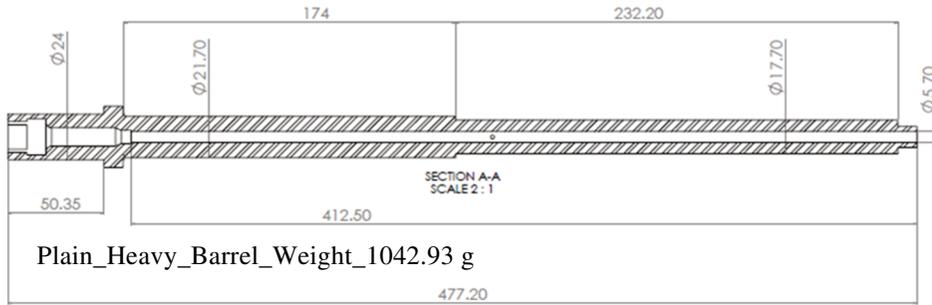
Fig. 1 Conventional machine gun barrel with thick mid-portion
