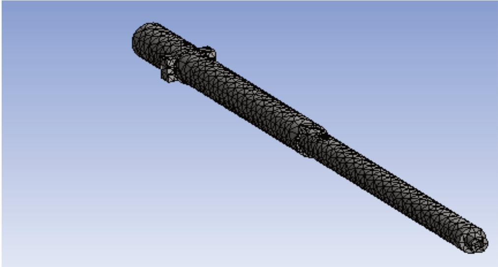
*Fig. 4 Mesh representation of the conventional barrel model*
