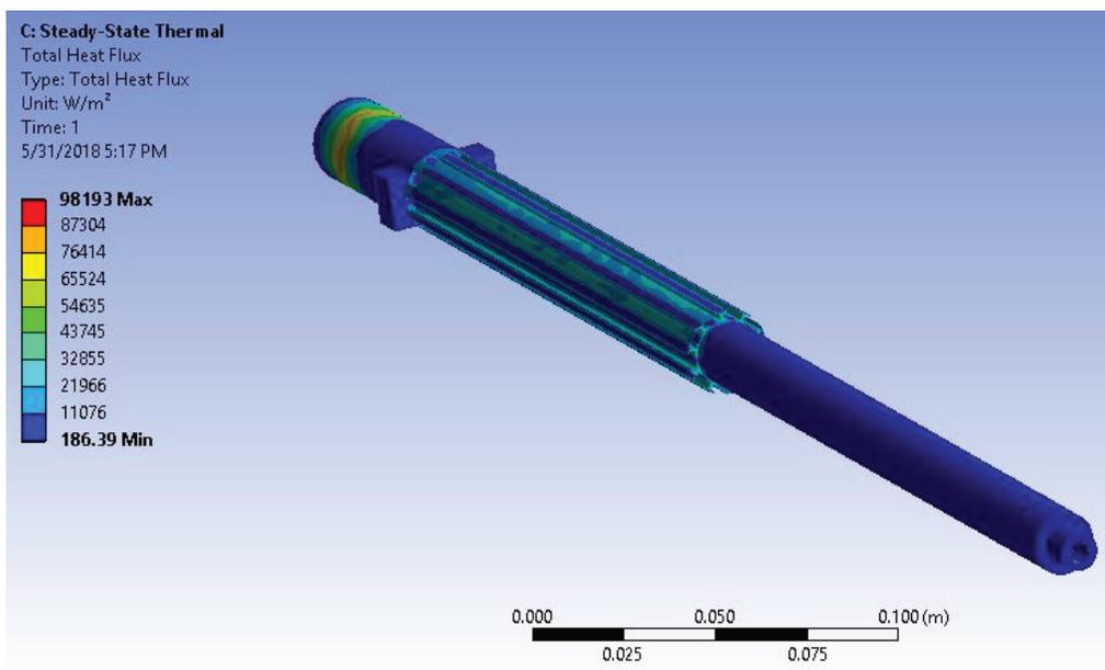
*Fig. 7 Enhancement in heat dissipation by T section fins*
