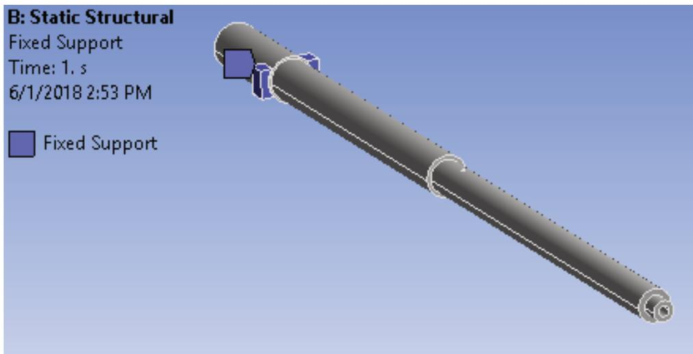
*Fig. 5 Fixed supports applied at the protruding lugs*
