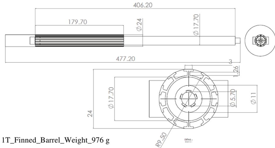
Fig. 2 Modified barrel with T-fins along the mid-length of the barrel
