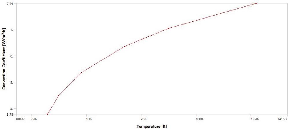
*Fig. 3 Atmospheric heat transfer coefficient variation with film temperature*
