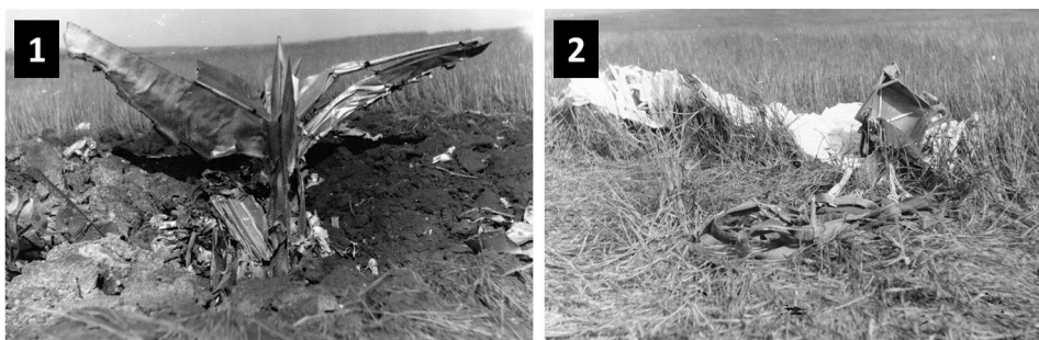
Fig. 1 The MiG-15 disaster – June 16 th , 1958: (1) tailplane debris, (2) KK-1 type ejection seat [17]
