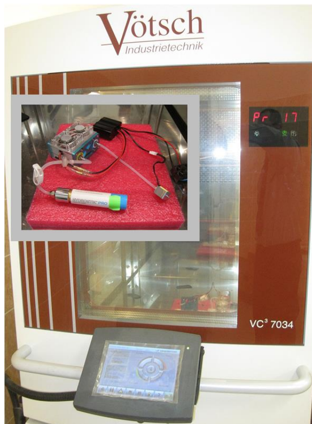
Fig. 3 Thermal chamber of the measuring station with the H-30 fuel cell
