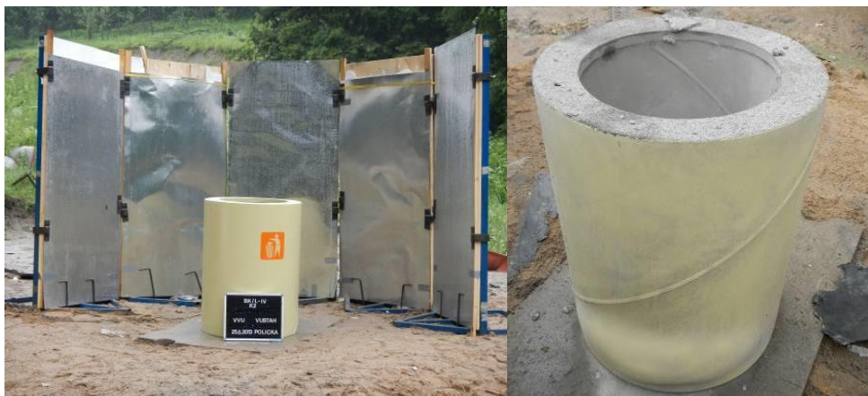
Fig. 7 Blast test layout (left) and element after the blast test (right)
