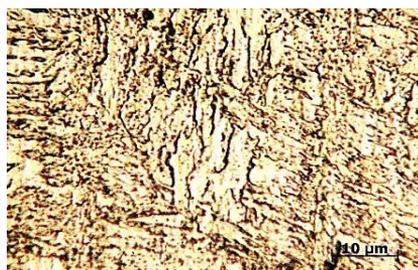
*Fig. 6 Widmanstätten-type structure inside weld*
