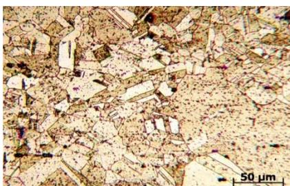
Fig. 7 Microstructure of flame tube
