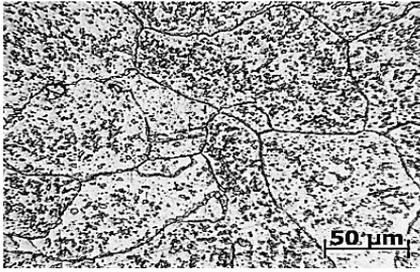
Fig.14 Outer ring material microstructure
