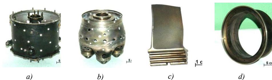
*Fig. 2 Analysed parts: a) combustion chamber casing, b) flame tube
