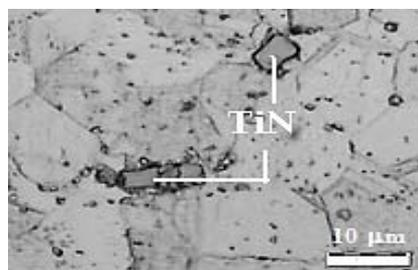
Fig 8 Precipitates – carbides and TiN
