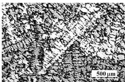
Fig. 9 Dendritic structure of blade
