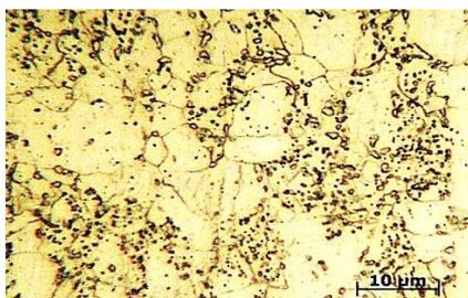
*Fig. 5 Ferritic-pearlitic structure with globular pearlite*
