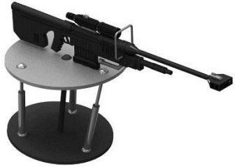
Fig. 7 Parallel robot used as sentry device
