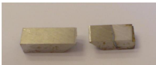
Fig. 1 Sample for evaluation of Ti coating thickness with V-notch after its fracture.
